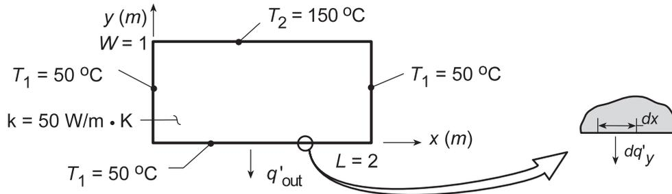
**ASSUMPTIONS:** (1) Two-dimensional, steady-state conduction, (2) Constant properties.
