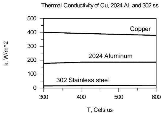
Note the large difference between the thermal conductivities of these metals. Copper conducts thermal energy effectively, while stainless steels are relatively poor thermal conductors. Also note that, depending on the metal, the thermal conductivity increases (2024 Aluminum and 302 Stainless Steel) or decreases (Copper) with temperature.
