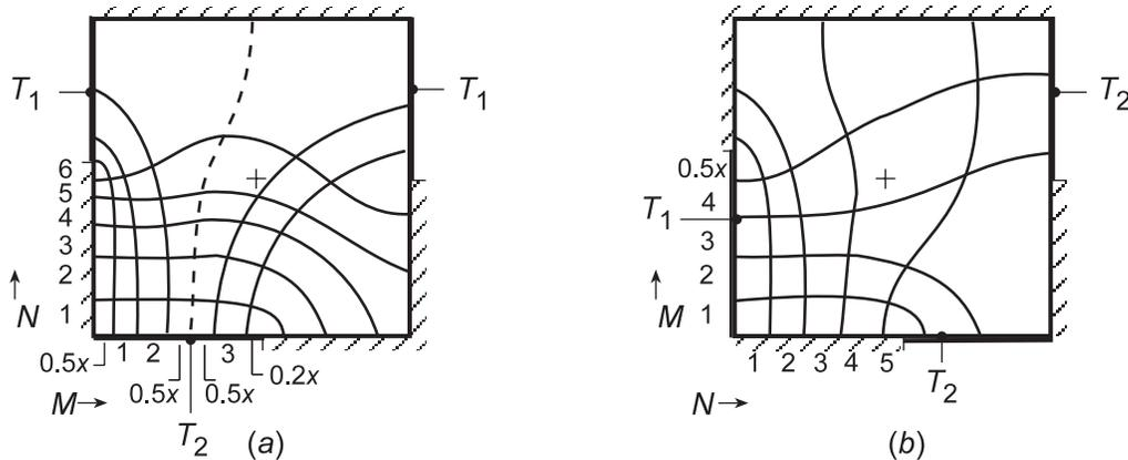
The shape factors are calculated from Equation 4S.7 and the heat rate from Equation 4S.6.
