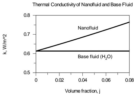
Note the increase in the thermal conductivity of the nanofluid with addition of more nanoparticles. The solid phase usually has a higher thermal conductivity than the liquid phase, as noted in Figures 2.5 and 2.9, respectively.
