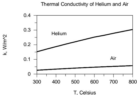
Note the high thermal conductivity of helium relative to that of air. As such, He is sometimes used as a coolant. The thermal conductivity of both gases increases with temperature, as expected from inspection of Figure 2.8.
