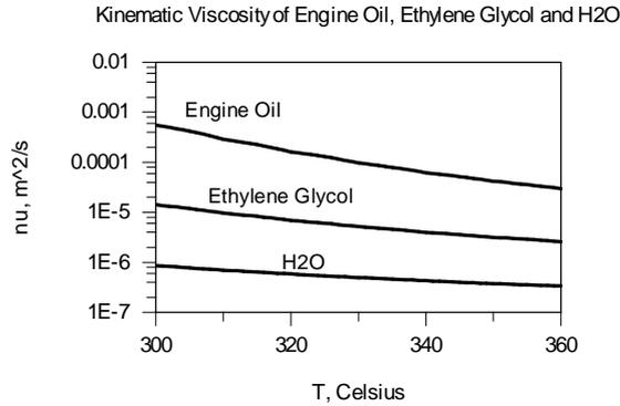
The kinematic viscosities vary by three orders of magnitude between the various liquids. For each case the kinematic viscosity decreases with temperature.
