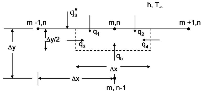
**ASSUMPTIONS:** (1) Two dimensional, steady-state conduction with no generation, (2) Constant properties.
