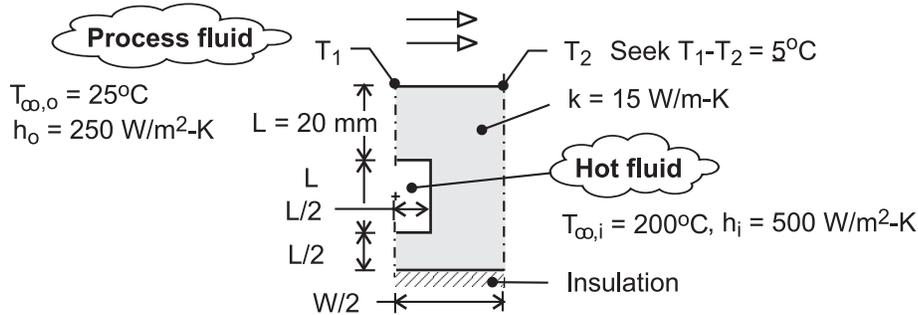
**ASSUMPTIONS:** (1) Steady-state, two-dimensional conduction with constant properties, and (2) Lower surface of platen is adiabatic.
