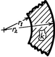
$$R_t = \frac{1}{4\pi k} \left[ \frac{1}{r_1} - \frac{1}{r_2} \right] \quad S = \frac{4\pi}{1/r_1 - 1/r_2} \quad <$$
