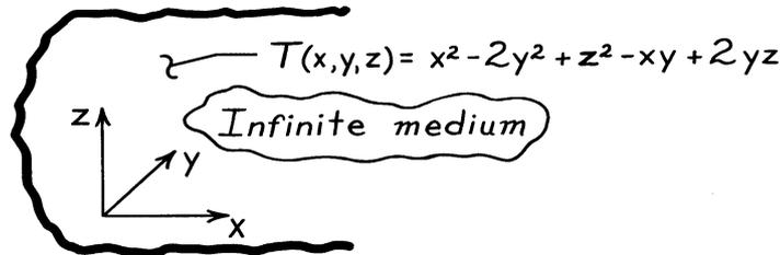
**ASSUMPTIONS:** (1) Constant properties of infinite medium and (2) No internal heat generation.
