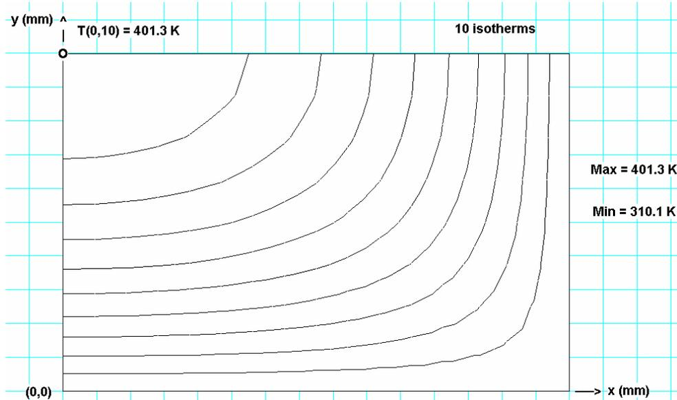
The isotherms are normal to the symmetrical lines as expected since those surfaces are adiabatic. The isotherms, especially near the center, have an elliptical shape. Along the  $x = 0$  axis and the  $y = 10$  mm axis, the temperature gradient is nearly linear. The hottest point is of course the center for which the temperature is
