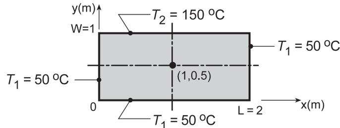
**ASSUMPTIONS:** (1) Two-dimensional, steady-state conduction, (2) Constant properties.
