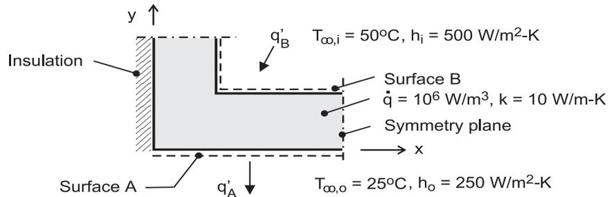
**ASSUMPTIONS:** (1) Steady-state, two-dimensional conduction, (2) Constant properties.
