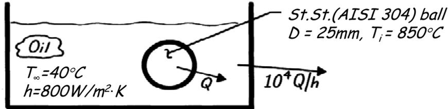
**ASSUMPTIONS:** (1) One-dimensional radial conduction in ball bearings, (2) Constant properties.
