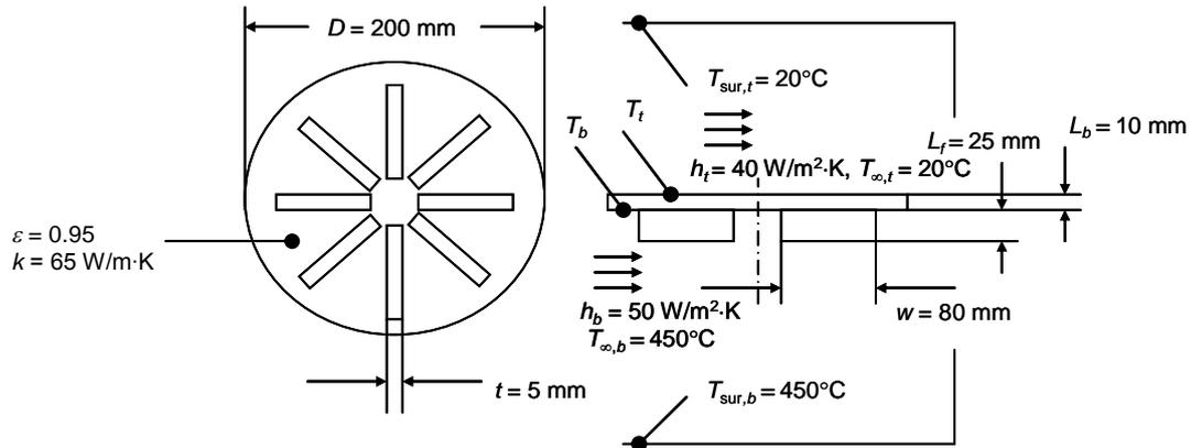
**ASSUMPTIONS:** (1) Steady-state, one-dimensional conditions, (2) Constant properties, (3) Convection from fin tip, (4) Large surroundings at top and bottom of burner.
