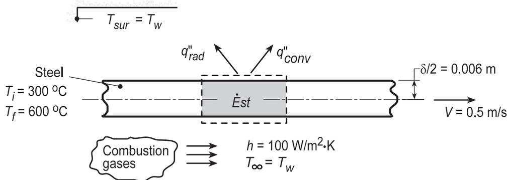
**ASSUMPTIONS:** (1) Constant properties, (2) Negligible temperature gradients in transverse direction across strip, (c) Negligible effect of strip conduction in longitudinal direction.
