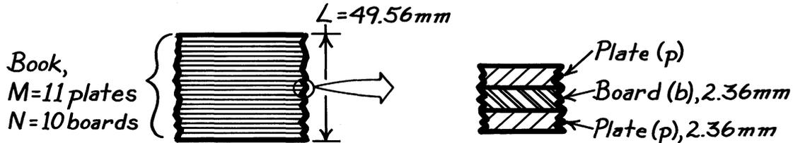
**ASSUMPTIONS:** (1) One-dimensional conduction, (2) Negligible contact resistance between plates and boards.
