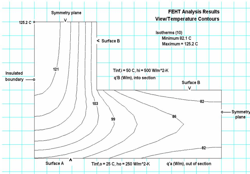
The hottest region of the section is the upper vertical leg (left-hand corner). The coolest region is in the lower horizontal leg at the far right-hand boundary. The maximum and minimum section temperatures (125°C and 77°C), respectively, are higher than either adjoining fluid. Remembering that heat flow lines are normal to the isotherms, heat flows from the hottest corner directly to the inner fluid and downward into the lower leg and then flows out surface A and the lower portion of surface B.
