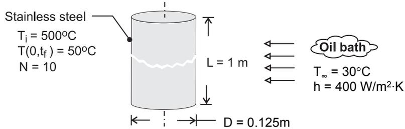
**ASSUMPTIONS:** (1) One-dimensional, radial conduction in rod, (2) Constant properties.
