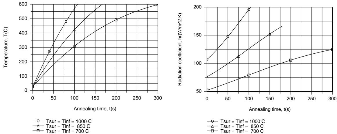
As expected, the heating rate and time, respectively, increase and decrease significantly with increasing  $T_w$ . Although the radiation heat transfer rate decreases with increasing time, the coefficient  $h_r$  increases with  $t$  as the strip temperature approaches  $T_w$ .
