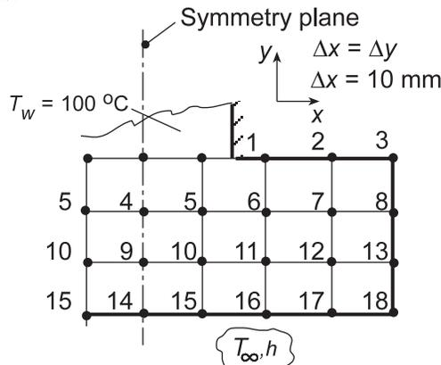
Using the *IHT Finite-Difference Equations Tool*, the set of nodal equations can be readily formulated. The temperature distribution ( $^\circ\text{C}$ ) is tabulated in the same arrangement as the nodal network.
