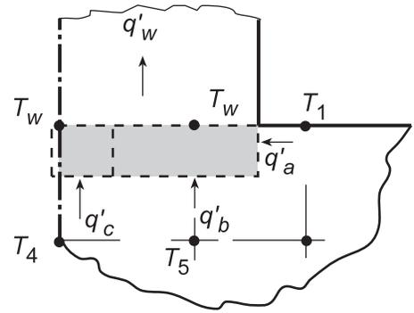
$$q'_w = 10 \text{ W/m} \cdot \text{K} [(215.8 - 100)/2 + (177.1 - 100) + (166.6 - 100)/2] \text{ K} = 1683 \text{ W/m} \quad <$$
