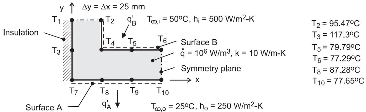
**ASSUMPTIONS:** (1) Steady-state, two-dimensional conduction, (2) Constant properties.
