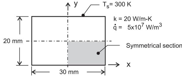
**ASSUMPTIONS:** (1) Steady-state conditions, and (2) Two-dimensional conduction with constant properties.
