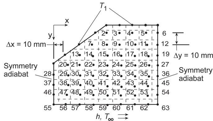
**ASSUMPTIONS:** (1) Steady-state, two-dimensional conduction, (2) Constant properties.
