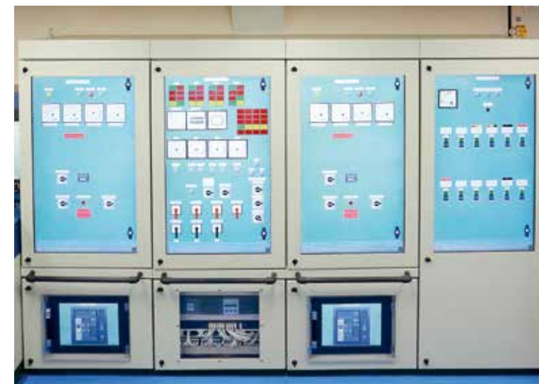
▲ 배전반 실습 콘솔 Switch Board Training Console
