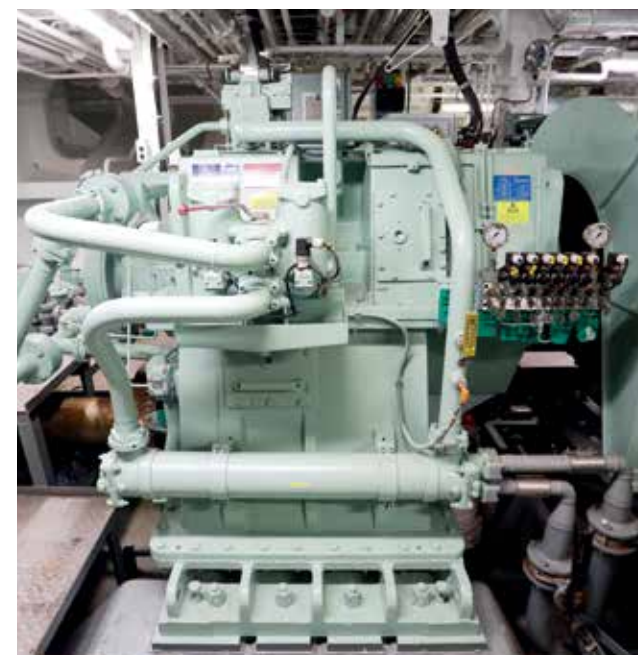
▲ 감속기 Reduction Gear
