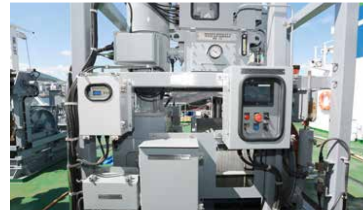
▲ MOCNESS 윈치 MOCNESS Winch (EM Cable 11mm / 2,000m)
