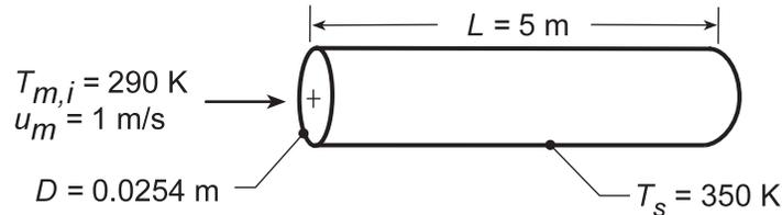
**ASSUMPTIONS:** (1) Negligible tube wall conduction resistance, (2) Incompressible liquid with negligible viscous dissipation.
