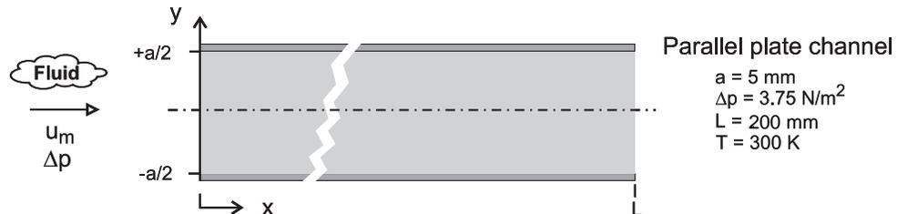
**ASSUMPTIONS:** (1) Fully developed laminar flow, (2) Parallel-plate channel,  $a \ll b$ .
