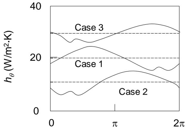
For Case 1,  $\bar{h} \approx 20$  W/m<sup>2</sup>·K; for Case 2,  $\bar{h} \approx 10$  W/m<sup>2</sup>·K, for Case 3,  $\bar{h} \approx 30$  W/m<sup>2</sup>·K <
