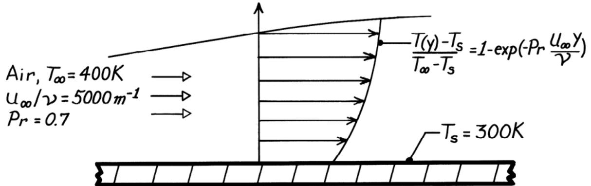
**PROPERTIES:** Table A-4, Air ( $T_s = 300\text{K}$ ):  $k = 0.0263\text{ W/m}\cdot\text{K}$ .
