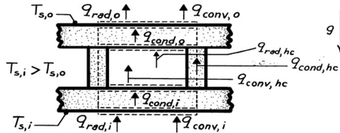
The above schematic represents the cross section of a single honeycomb cell and surface slabs. Assumed direction of gravity field is downward. Assuming that the bottom (inner) surface temperature exceeds the top (outer) surface temperature ( $T_{s,i} > T_{s,o}$ ), heat transfer is in the direction shown.
