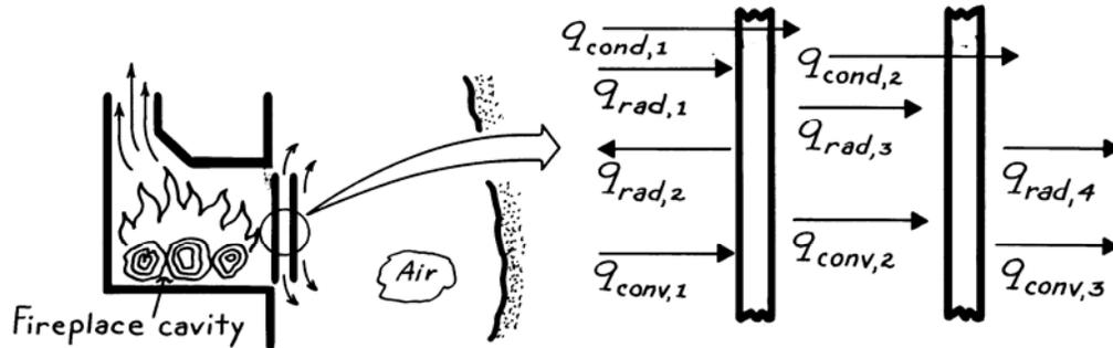
The relevant heat transfer processes associated with the double-glazed, glass fire screen are:
