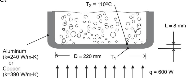
**ASSUMPTIONS:** (1) One-dimensional, steady-state conduction through bottom of pan.
