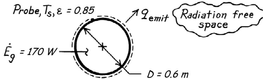
**ASSUMPTIONS:** (1) Steady-state conditions, (2) Negligible radiation incident on the probe.
