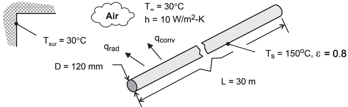
**ASSUMPTIONS:** (1) Steam line operates continuously throughout year, (2) Net radiation transfer is between small surface (steam line) and large enclosure (plant walls).
