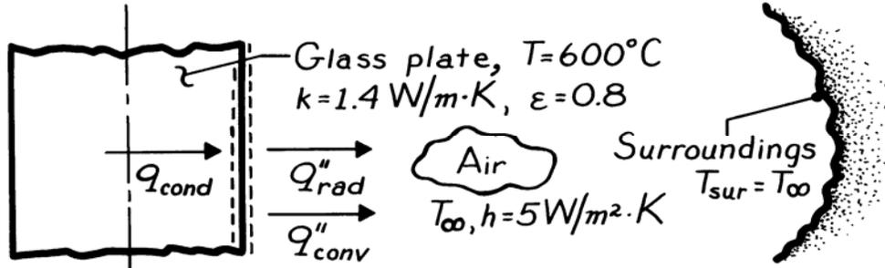
**ASSUMPTIONS:** (1) Surface of glass exchanges radiation with large surroundings at  $T_{\text{sur}} = T_\infty$ , (2) One-dimensional conduction in the  $x$ -direction.
