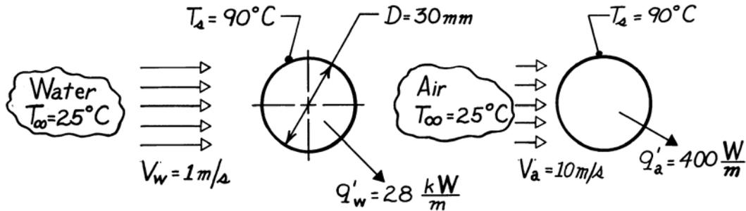
**ASSUMPTIONS:** (1) Flow is cross-wise over cylinder which is very long in the direction normal to flow.
