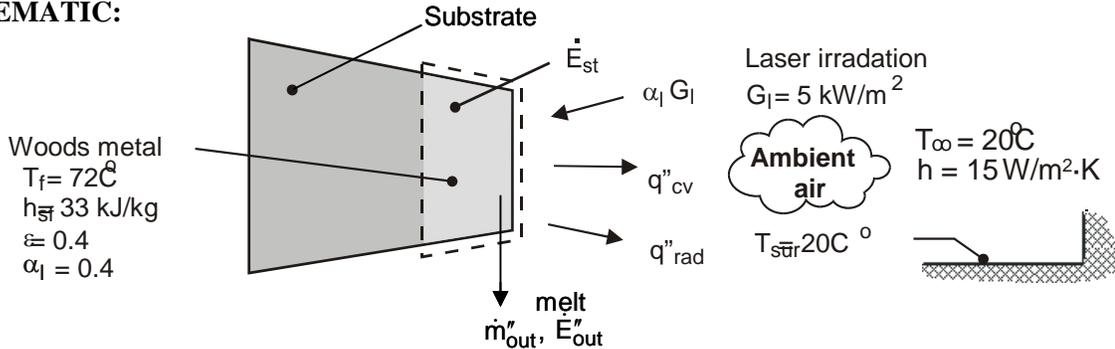
**ASSUMPTIONS:** (1) Woods metal slab is isothermal at the fusion temperature,  $T_f$ , and (2) The melt runs off the irradiated surface.
