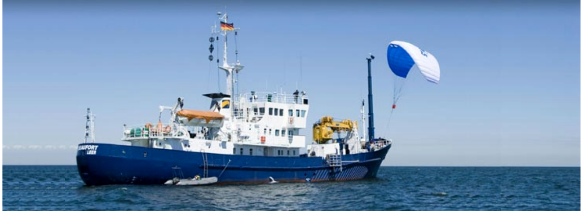
Fig. P7.89. Ship propulsion assisted by a large kite. [Copyright SkySails, Inc.]
