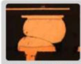
Cross Section analysis of solder ball non-wetting High Power Scope Analysis
