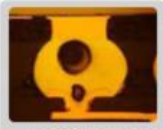
Cross Section analysis of solder void High Power Scope Analysis
